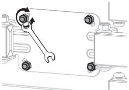
**Note:** Adjust the screws as shown to level the display.
