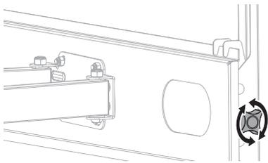
**Note:** Adjust to the desired angle and then tighten the knobs as shown.
